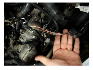
To adjust the Nissan TPS if its out of adjustment, watch the resistance from black to white - adjust it to be as low as possible. The Toyota ECU seems to accept a very wide range of values as normal, so adjustment may not be necessary.
