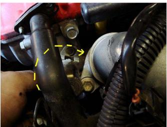
**Step 24** – Remove the 5 12mm fasteners securing the intake manifold to the cylinder head
