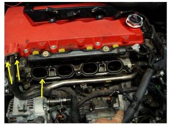
**Step 39** – Using a razor carefully cut the electrical tape off of the vertical portion of the wiring harness loom to gain access to the wires. Pull the IAC and TPS wires out from the rest of the harness down to the transition to horizontal on the harness.
