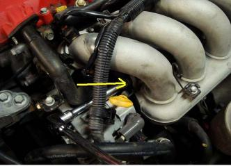
**Step 21** – Pull breather tube back away from head as far as it can go. (do not force it or pull it all the way off the studs.
