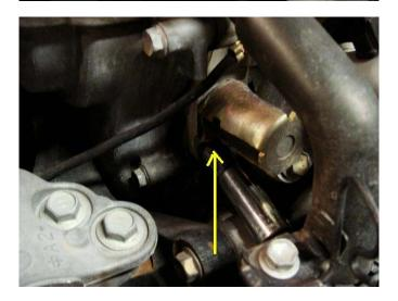
**Step 19** – Remove the 2 10mm nuts securing the crankcase breather tube to the valve cover.
