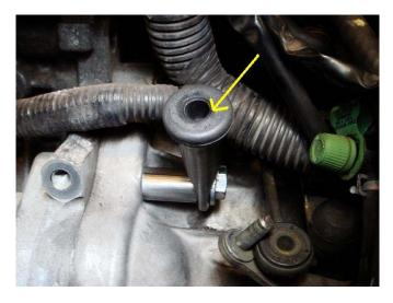
**Step 37** – Install dipstick tube standoff as shown. It will be necessary to rotate the dipstick tube counterclockwise to provide proper clearance to the intake runners. Please be sure to use the nylock (The M8 lock nut provided) on the end of the standoff.
