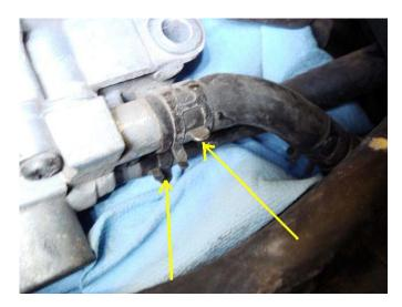
**Step 30** – Remove stub hose from thermostatic valve and valve to the other hose from the throttle body.
