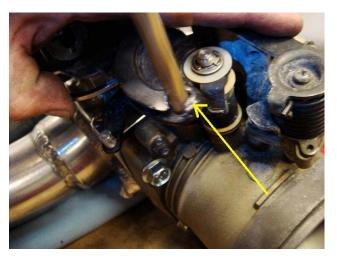
**Step 49** – Install the throttle body to the DD Performance Research Intake Manifold Utilizing the 4 M8 bolts and 4 M8 washers (provided).
