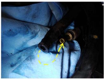
**Step 31** – Remove coolant reservoir lower mounting grommet from mounting bracket by fans.
