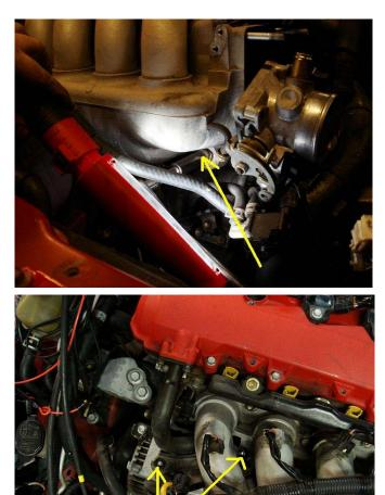
**Step 18** – Remove the 10mm bolt securing the VVTi OCV to the cylinder head.
